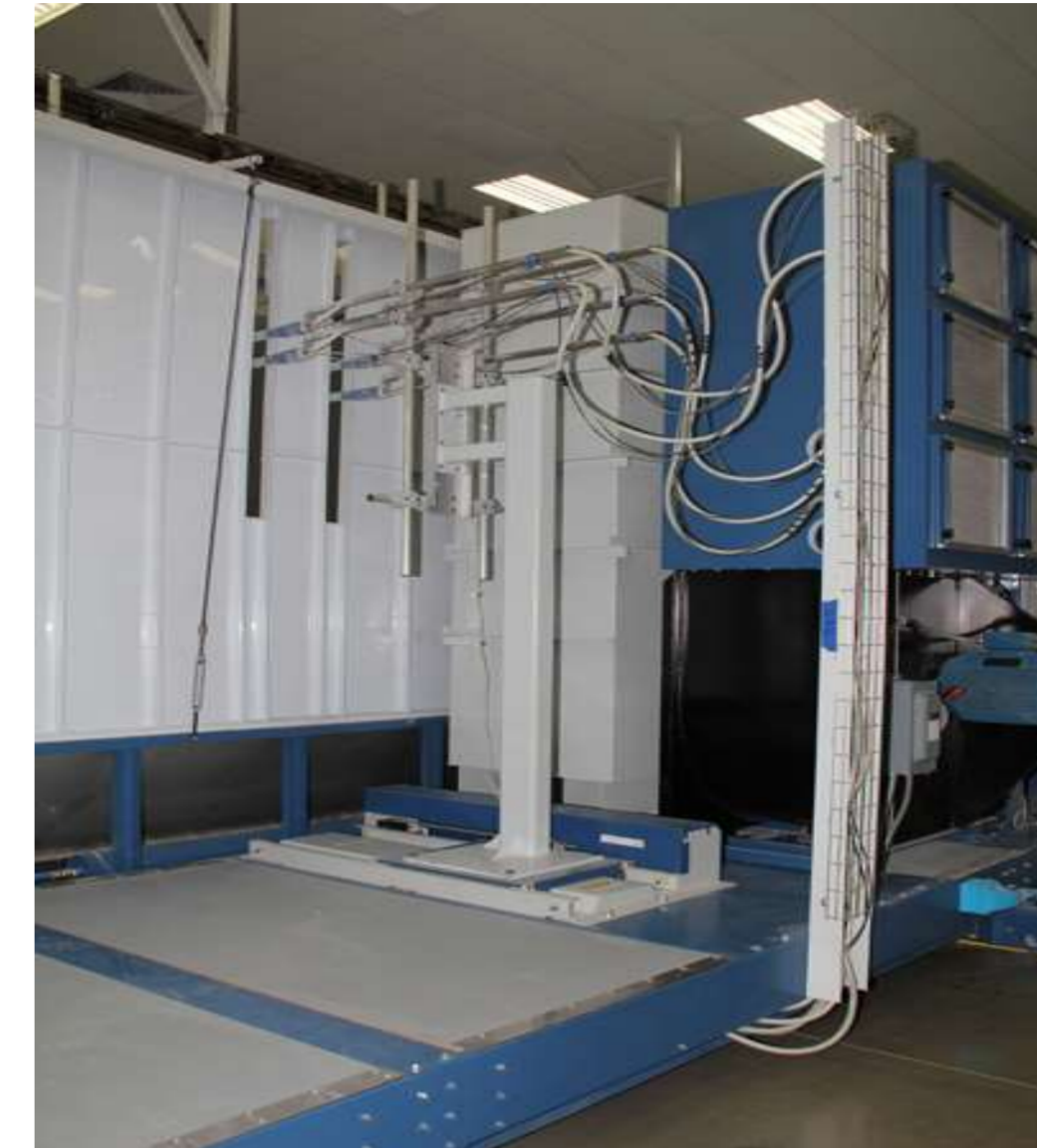
Six fixed gun stands with in-out positions.
