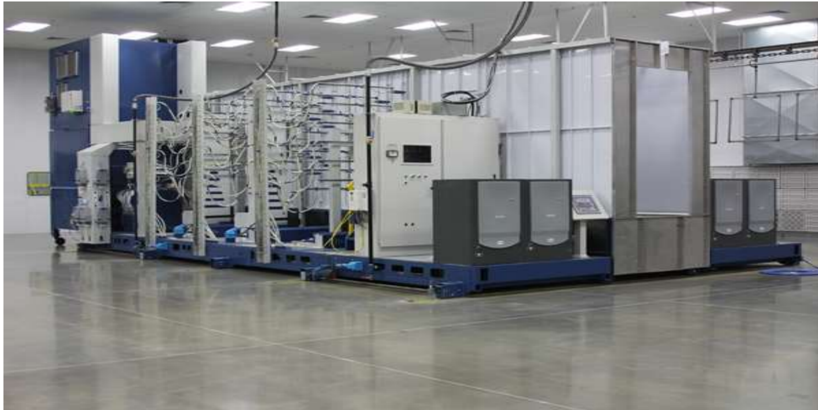
Six fixed gun stands with in-out positions.
