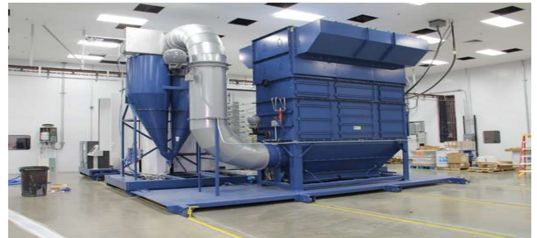
Booth moves off-line to change colors.
