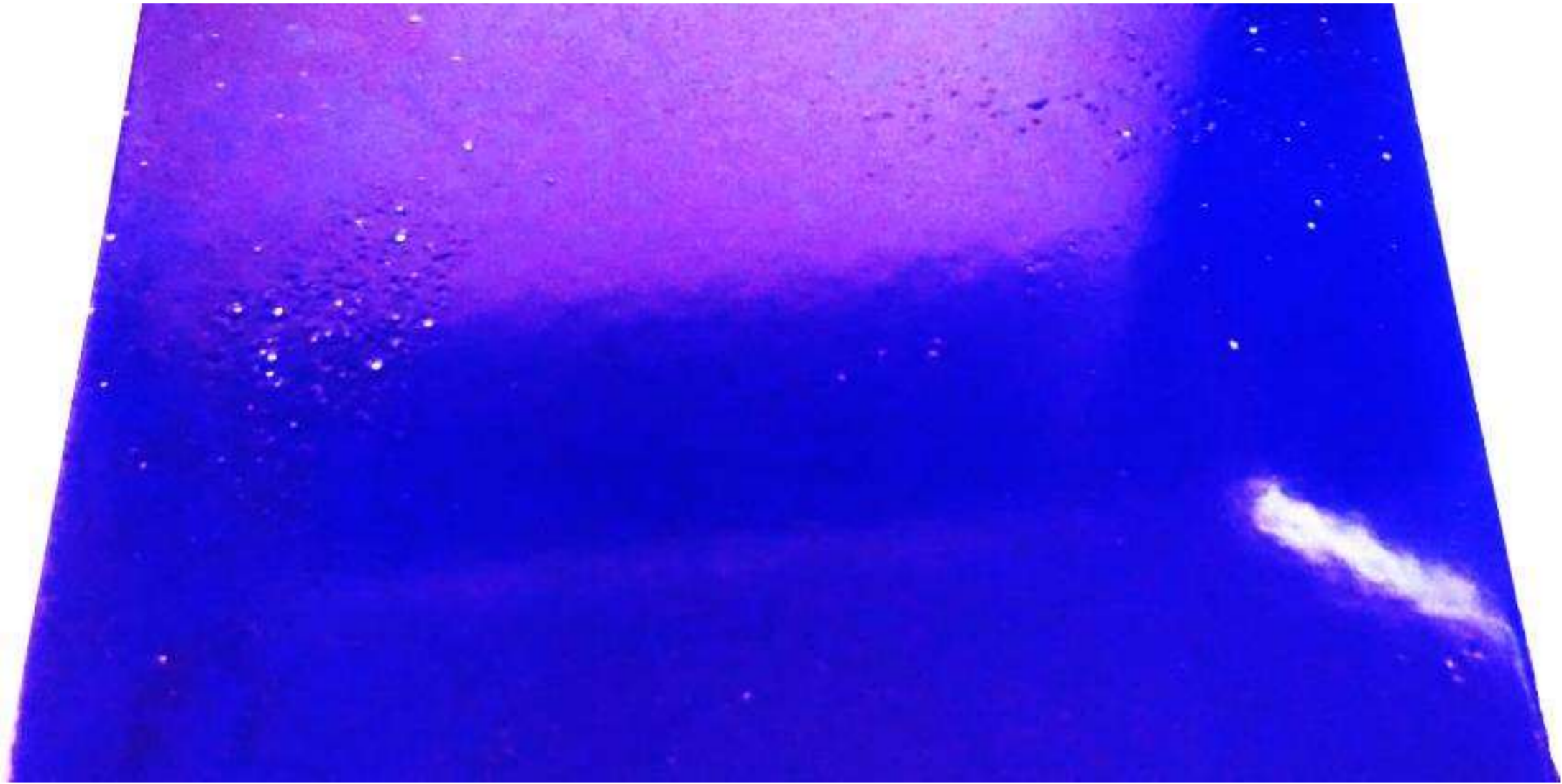
Enamel defects due to mill scale
