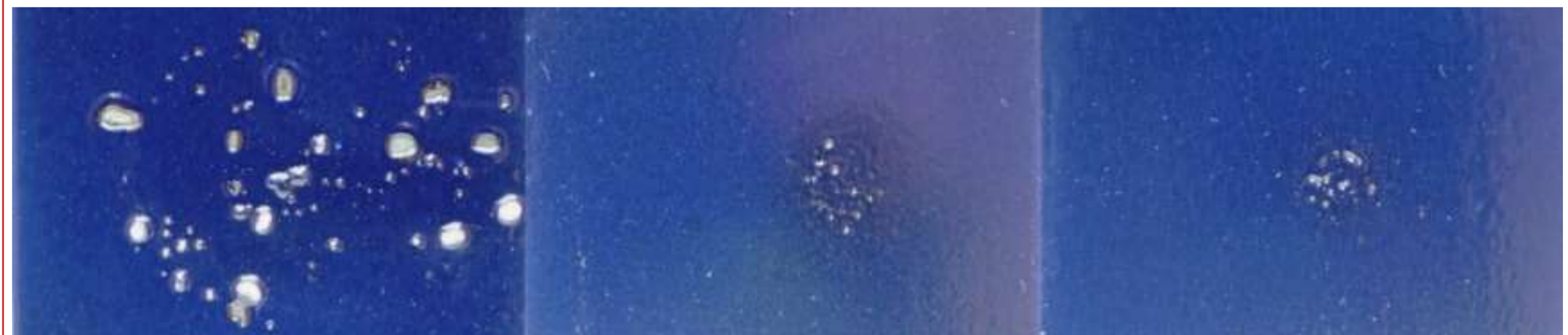
Improper rinsing ...base residues (up) or acid residues (below)
