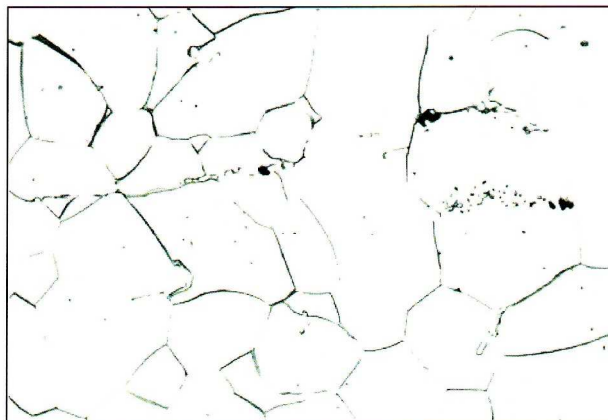
Fig. 12 The microstructure of hot rolled DC04 EK-B grade sample (nital, 500x)
